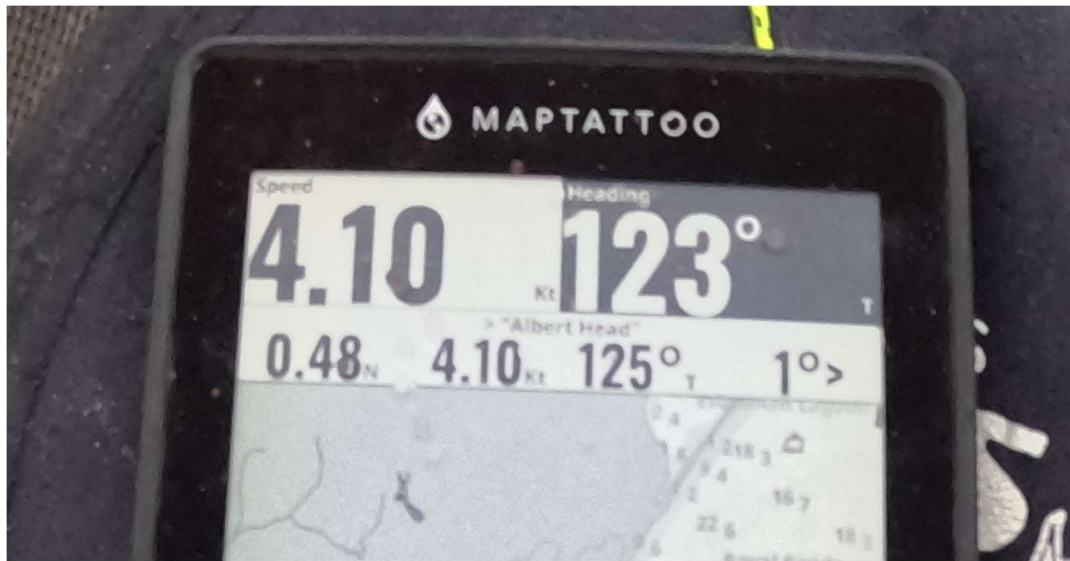
Figure 2. The basic speed and heading display and custom navigation bar
